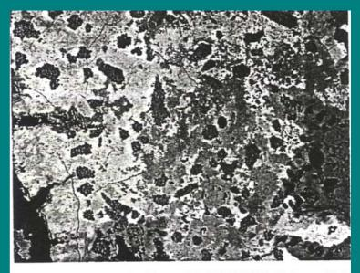
Fig. 8: Fatmalı-Kalecik, litharge No. TR 24/7. Inclusions of silver in lead oxide. Small black spots of silver chloride are scattered on the silver metal (gray). According to EDX measurements, the Ag concentrations in the lead oxide are slightly higher nearby these inclusions then in other parts of the litharge cake. Electron micrograph, BSE image. Length of image about 0.41 mm.
